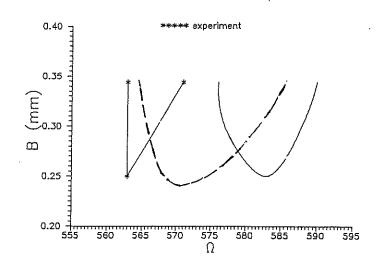
Figure 1: Stability diagram: a) Linear damping model without noise (top). b) non-linear damping model with and without weak noise (bottom).
