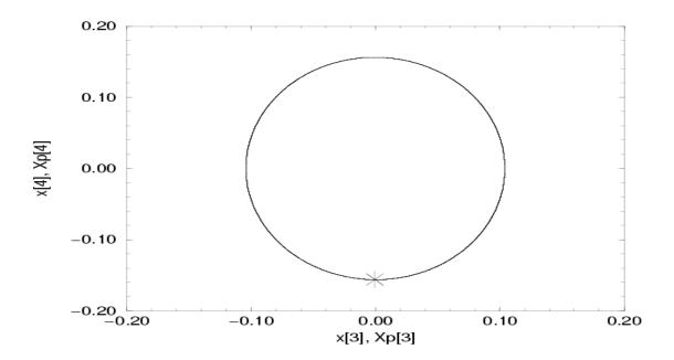
Fig 3 Modulated response of the actuated element (  $\alpha$  = 0.12,  $\mu$  = 0.8448,  $\beta$  = 0.01,  $\gamma$  = 0.05,  $\Omega_1$  = 1.5): state space (dy/dt(y), y=x[3], dy/dt=x[4]) and Poincare' map (Xp[4](Xp[3])) for a)  $\Omega_2$  = 0.7, b)  $\Omega_2$  = 3.0.
