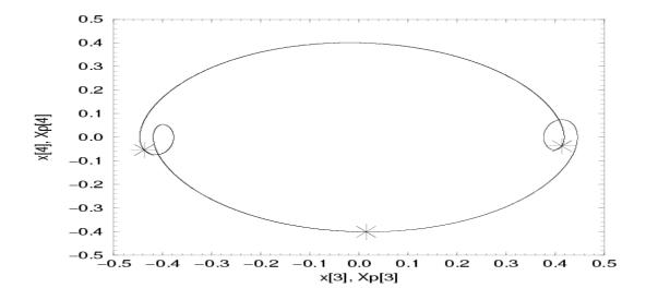
Fig 1 Third subharmonic response without element actuation (  $\Omega_1$  = 1.5 ): state space (dy/dt(y), y=x[3], dy/dt=x[4]) and Poincare' map (Xp[4](Xp[3])) for a)  $\alpha$  = 1/3,  $\mu$  = 0.5926, b)  $\alpha$  = 0.12,  $\mu$  = 0.8448.
